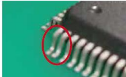
Lead float defect
